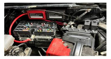
**12.** Using a pair of side/diagonal cutters, cut a 15mm deep notch into the fuse panel cover in the location shown in the images below. This notch is necessary to provide clearance for the positive battery cable previously installed in step 7.
