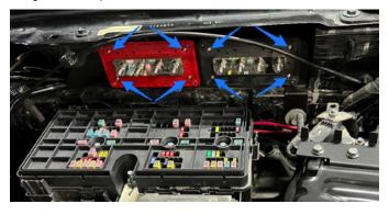
**7.** Fasten one side of the positive battery cable to the rearmost terminal post on the positive bus bar and the other side to the fuse panel terminal post.
