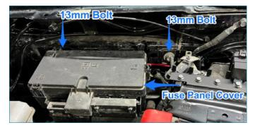
Feed the bus bar bracket into the drive-side of the engine bay and set the rearward mounting point onto the rear 13mm bolt.
