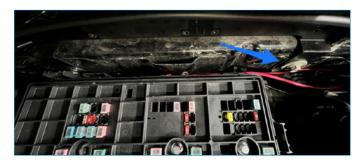
Tighten the 13mm bolts to secure the bus bar bracket.
