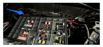
**3.** Rotate the front of the bus bar bracket upward and inward towards the side of the engine bay and then lower it onto the front 13mm bolt.
