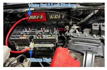
**B.** Fasten one side of the negative battery cable to the forward-most terminal post on the negative bus bar and the other side to the chassis ground.
