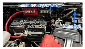
**9.** Connect all Borne Off-Road lighting/accessory positive and negative ring terminals to the remaining bus bar terminal posts.
