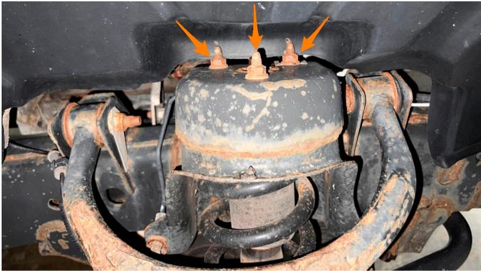
**09.** Using a pry bar, remove the strut by prying between the strut and the control arm. Pry down on the arm, up on the strut, and pull the strut outward toward you.
