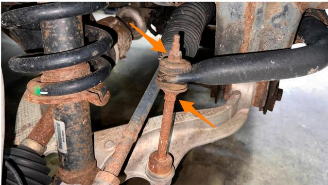
**05.** Using a 21mm wrench, remove the tie rod end nut. Counter-hold the threads using a 10mm socket. Loosely reinstall the nut so that the top of the nut is flush with the end of the threads. Using a hammer, hit the end of the threads to remove the tie rod end from the knuckle. [\[Image on top right\]](#)
