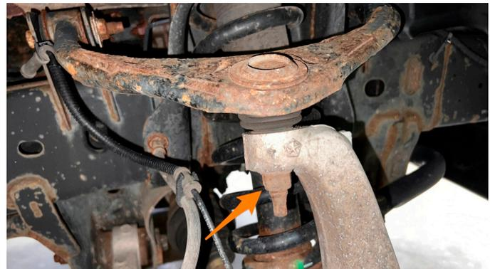
**07.** Hook the tie rod on the sway bar to keep out of the way. Remove the lower strut nut and bolt using a 21mm socket and 21mm wrench.
