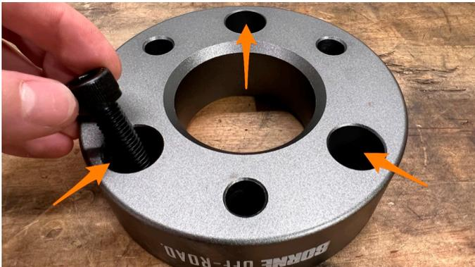
**11.** Fit the spacer onto the top of the strut. It will only go on in one orientation. Using a 17mm socket, install the spacer using the supplied M10 washers and lock nuts. Use a pry bar against the threads to keep the strut from rotating while tightening the nuts.
