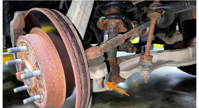
**06.** Using a 21mm wrench, remove the upper control arm ball joint nut. Counter-hold the threads using a 10mm socket. Loosely reinstall the nut so that the top of the nut is flush with the end of the threads. Using a hammer, hit the end of the threads to remove the tie rod end from the knuckle.
