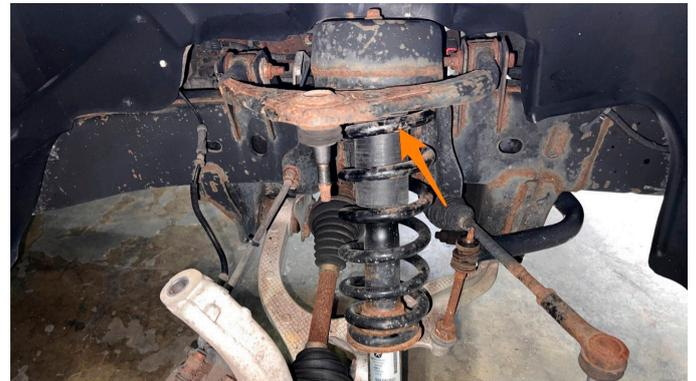
**13.** Pry down on the lower control arm until you can get the bottom of the strut over the front of the control arm and the bushing. Then, reinstall the lower strut nut and bolt.
