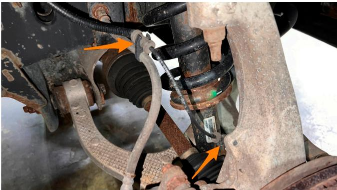
**04.** Using a 17mm socket, remove the upper sway bar link nut. Counter-hold the rod with a 15mm wrench.
