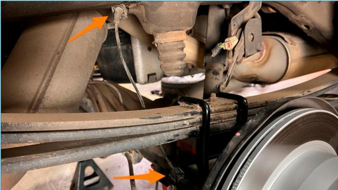
**03.** Use a pick tool to remove the ride height sensor pigtail on the driver's side.
