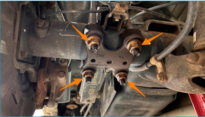
**09.** Using the floor jack, raise the frame of the truck on the side you're working on until you can remove the factory spacer block between the spring and the axle. Install the 2-inch spacer in its place, then carefully lower the truck back down onto the axle being sure the alignment pins on the spring/spacer fall in the corresponding holes.
