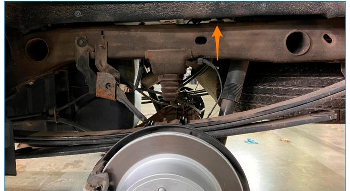
**06.** Using a 13mm socket, remove the bolt for the brake line bracket on top of the differential housing.
