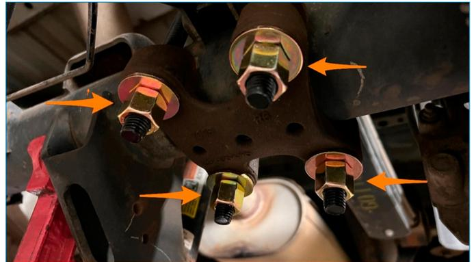
**12.** Reinstall the lower shock bolt and repeat steps 7-12 on the other side.
