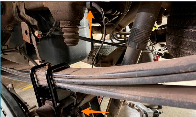
**04.** Using a 13mm socket, remove the bolt for the parking brake cable bracket on the driver's side and let the bracket hang free.
