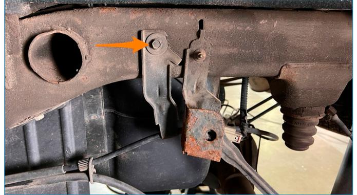
**05.** Using a 13mm wrench, remove the two bolts for the upper brake line bracket. These are on top of the frame rail on the driver's side.
