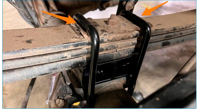
**11.** Using the supplied nuts and washers, install the lower support bracket and tighten using a 21mm deep socket to factory torque specifications.
